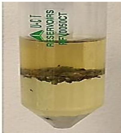
Figures 2 and 3: Recreational marijuana sample following QuEChERS extraction; Comparison of QuEChERS extracts before (left) and after (right) dSPE cleanup.
